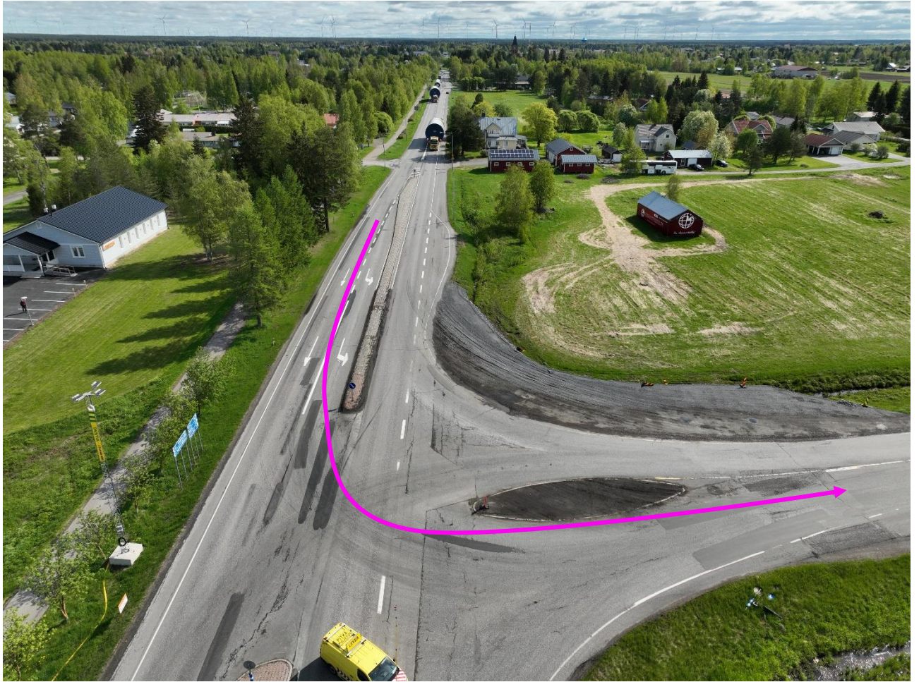
Turning from highway E8 to highway VT27 in Kalajoki has been modified for wind power transports.
